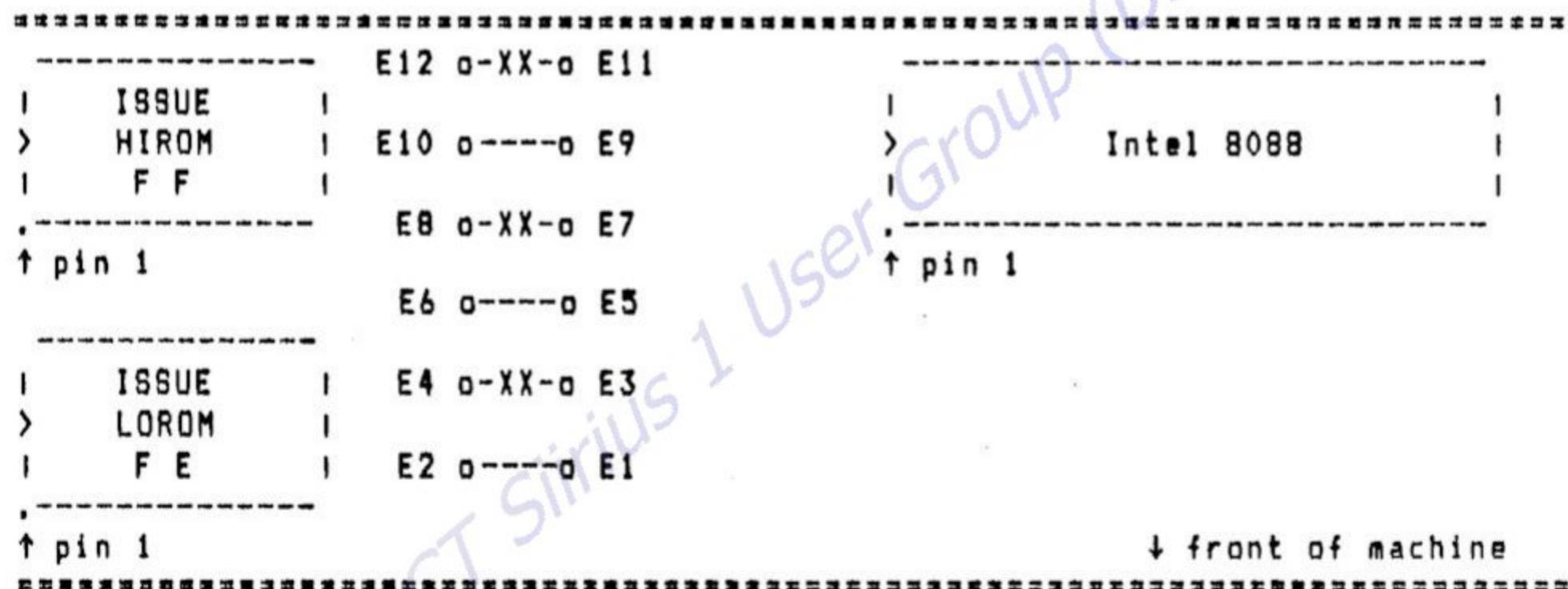
**IF TWO ROMS WERE FITTED,** or if the conversion from one ROM has been completed, fit the new Issue ROMs as shown above. Take care to ensure that each ROM is inserted into the correct socket, that pin 1 of each ROM is to the left of the machine and that no pins are sitting outside of the sockets. If all is correct, reassemble the machine and remake all connections.
